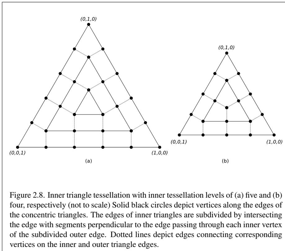
non-overlapping triangles as described above. If the first (and only) inner triangle is degenerate, a set of triangles is produced by connecting each vertex on the outer triangle edges with the center point.
