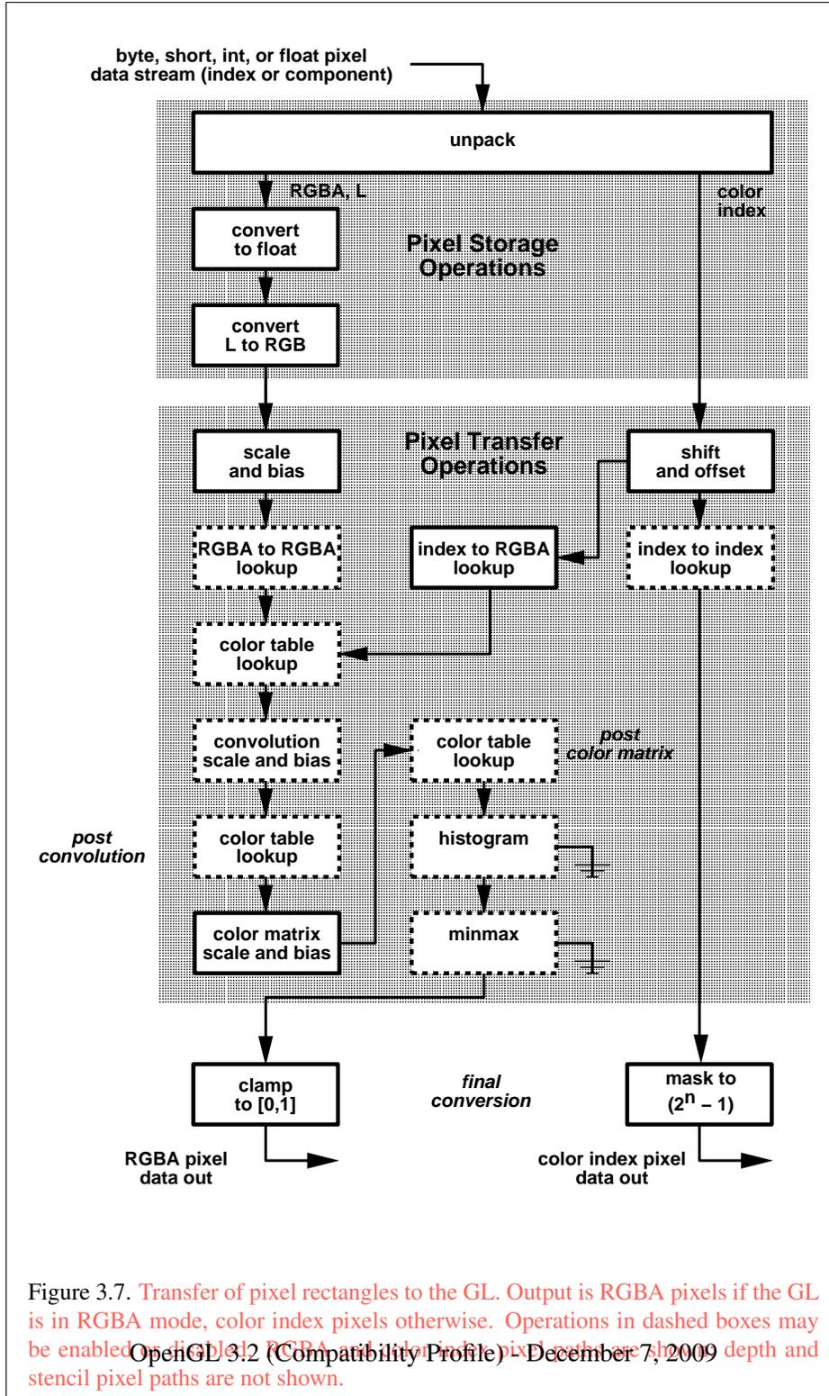
Figure 3.7. Transfer of pixel rectangles to the GL. Output is RGBA pixels if the GL is in RGBA mode, color index pixels otherwise. Operations in dashed boxes may be enabled on GL 3.1 (RGBA and color index pixel paths are shown).
