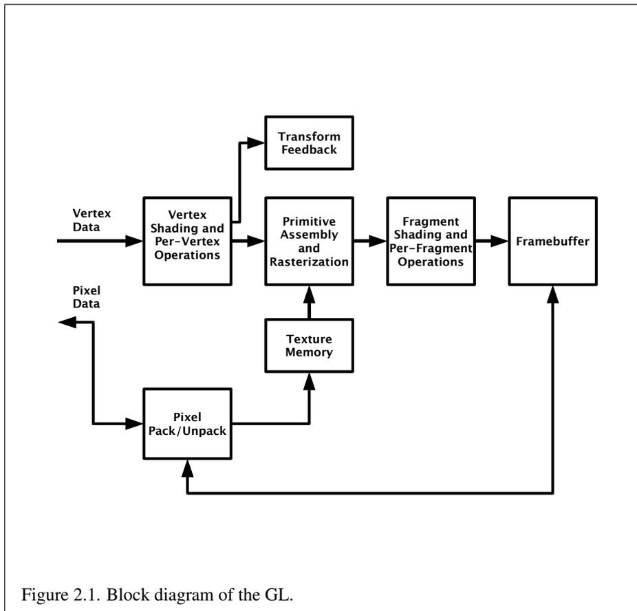
Figure 2.1. Block diagram of the GL.
