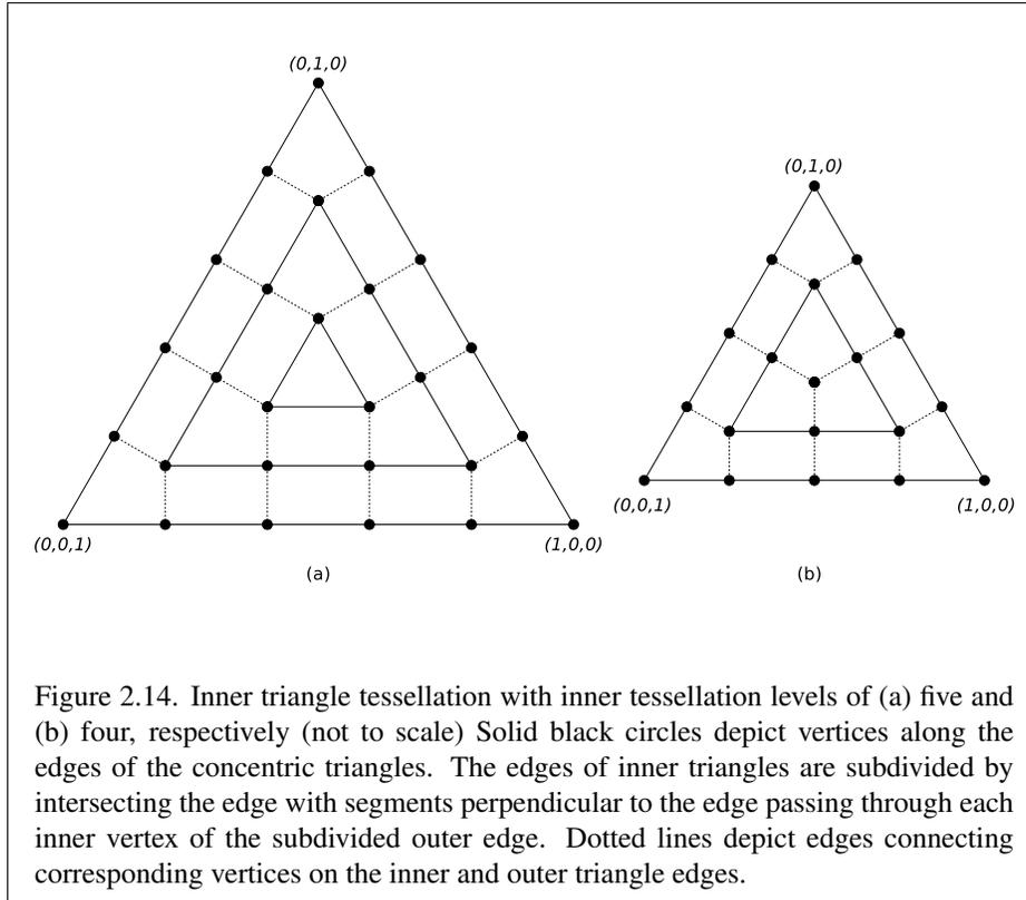
Figure 2.14. Inner triangle tessellation with inner tessellation levels of (a) five and (b) four, respectively (not to scale) Solid black circles depict vertices along the edges of the concentric triangles. The edges of inner triangles are subdivided by intersecting the edge with segments perpendicular to the edge passing through each inner vertex of the subdivided outer edge. Dotted lines depict edges connecting corresponding vertices on the inner and outer triangle edges.
