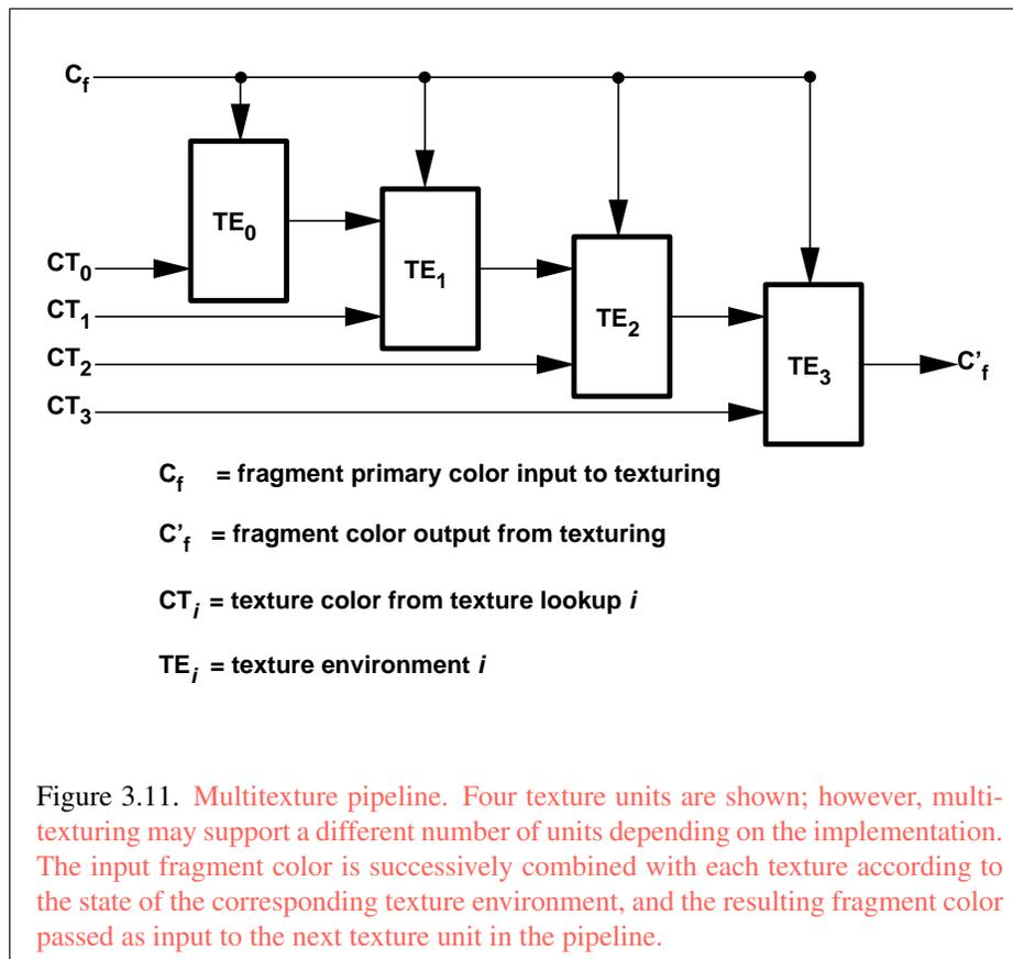
Figure 3.11. Multitexture pipeline. Four texture units are shown; however, multitexturing may support a different number of units depending on the implementation. The input fragment color is successively combined with each texture according to the state of the corresponding texture environment, and the resulting fragment color passed as input to the next texture unit in the pipeline.
