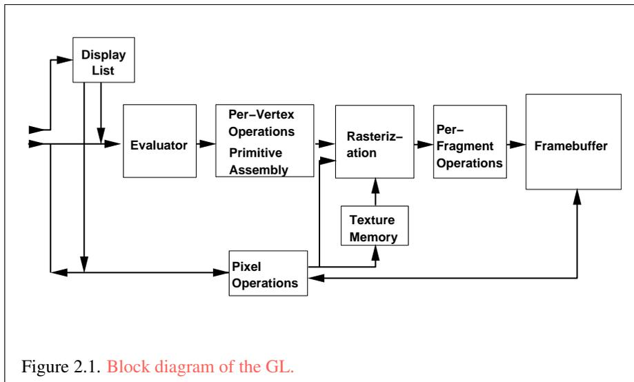
Figure 2.1. **Block diagram of the GL.**
